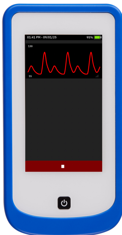
Figur 4-6: HemoSphere Stream™ modulets aktive bølgeformstransmission
