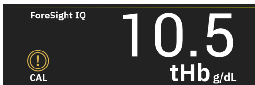
Figure 12-19: tHb parameter recalibration warning
