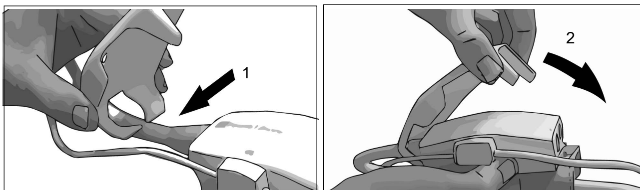
Figure B-1 Applying pressure controller cover
