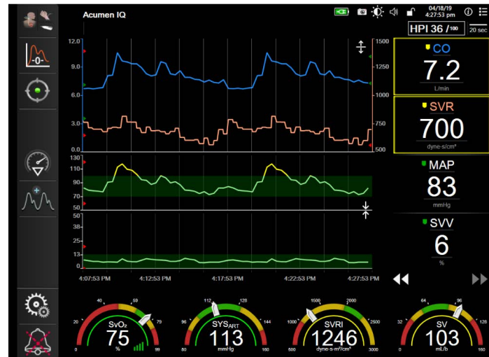
Figure 5-6 Main monitoring view
