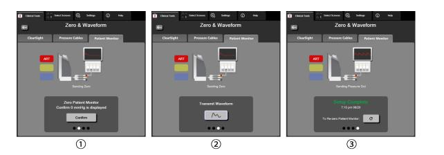
Figure 11-8: Transmit arterial pressure waveform to patient monitor
