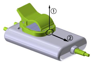
Figure 13-7: Removing the mounting clip
