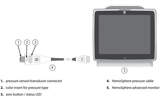
Figure 4-2: Pressure cable connection overview
