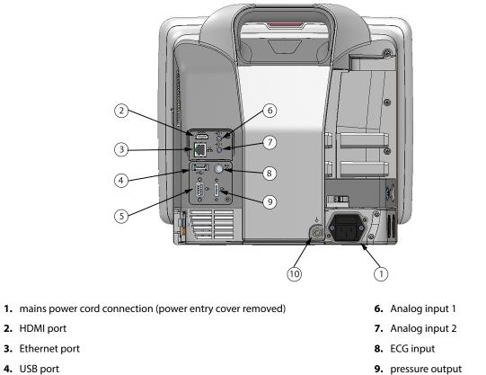
5. COM1 serial port connector (RS-232)
