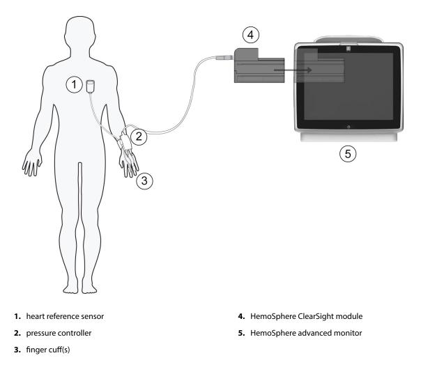
*Figure 4-5: HemoSphere noninvasive system connection overview*
