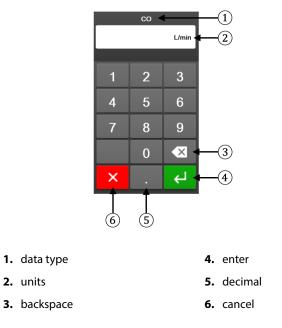
Keypad. Touch the keys on the keypad to enter numeric data.
