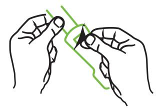
Figure 13-10: Removing protective liner from sensor
