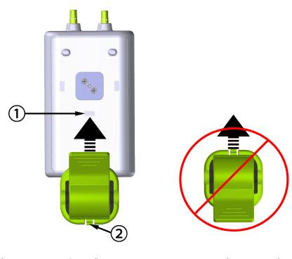
**1.** mounting clip retaining recess (vertical)
