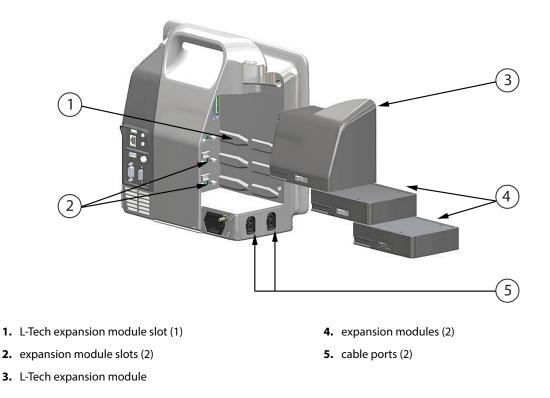
Figure 1-1: HemoSphere advanced monitor hemodynamic technology connections
