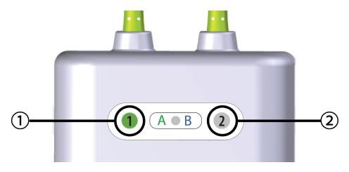
**1.** channel 1 LED is green (sensor connected)
