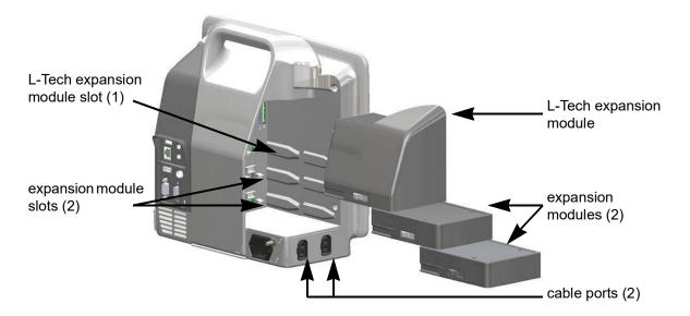
Figure 1-1 HemoSphere advanced monitor hemodynamic technology connections
