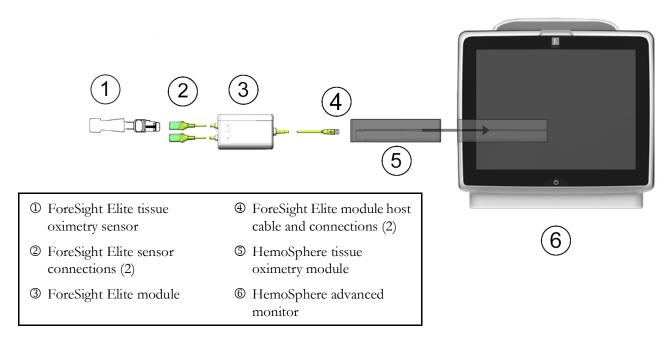
Figure 12-8 HemoSphere tissue oximetry module connection overview
