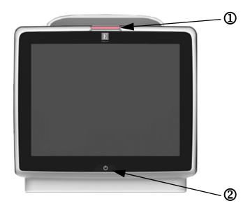
Figure 14-1 HemoSphere advanced monitor LED indicators
