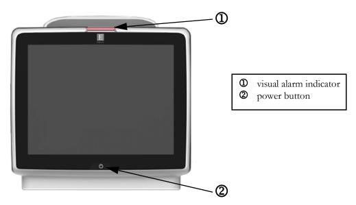
Figure 3-1 HemoSphere advanced monitor front view
