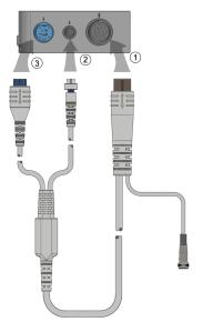
Figure 9-2 Patient CCO cable test connections
