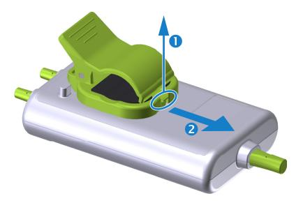
Figure 12-7 Removing the mounting clip
