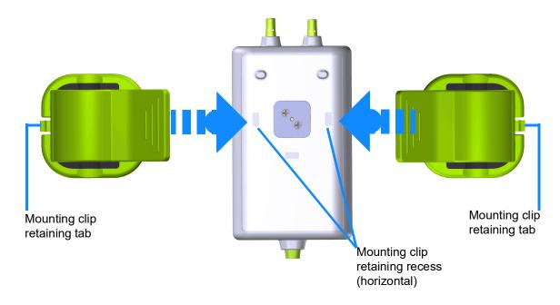
Figure 12-6 Attaching the mounting clip horizontally
