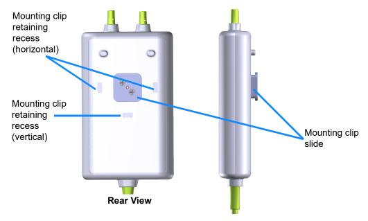
Figure 12-4 Module case – mounting clip attachment points
