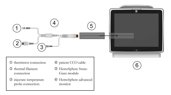
Figure 4-1 HemoSphere Swan-Ganz module monitoring connection overview
