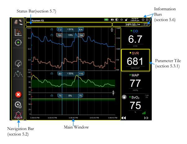
Figure 5-1 HemoSphere advanced monitor screen features
