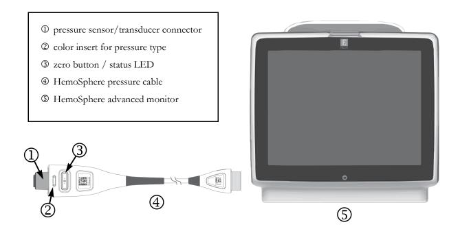
Figure 4-2 Pressure cable connection overview
