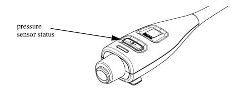
Figure 14-2 Pressure cable LED indicator
