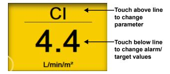
Figure 5-20 Focused parameter tile – parameter and alarm/target selection
