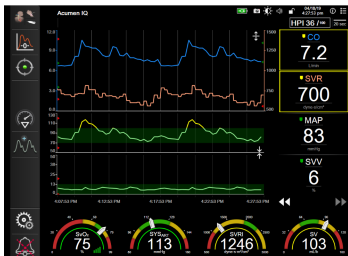
Figure 5-6 Main monitoring view
