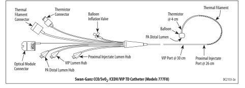
computer to continuously measure cardiac output. Models 744F75, 746F8, 774F75, and 777F8 also measure mixed venous oxygen saturation.
